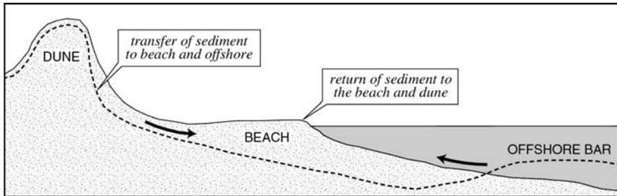
Fig. 2.1. Exchange of sand within the sand-sharing system
