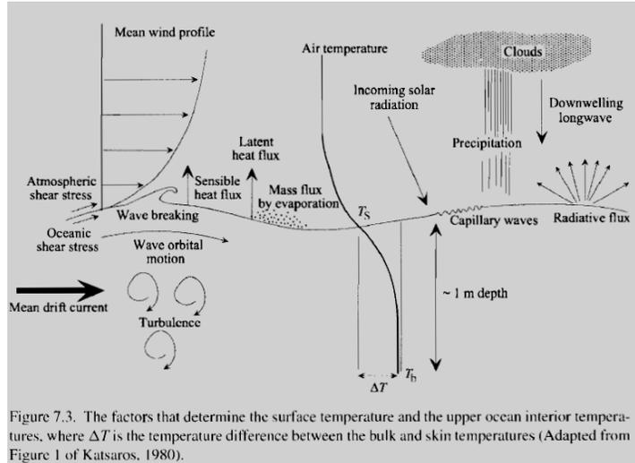
Figure 7.3. The factors that determine the surface temperature and the upper ocean interior temperatures, where  $\Delta T$  is the temperature difference between the bulk and skin temperatures (Adapted from Figure 1 of Katsaros, 1980).
