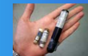
Fig. 6. Bluefish and Striped Bass tags, from left to right model: CAFT8-5, CAFT11_2, CAFT16_3. The bigger the tag the stronger the signal.
