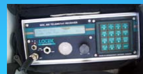
Fig. 5. The SRX displaying bass code 186 at a power of 207, meaning the bass is very close!
