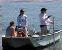
Figure 1B: Mobile tracking. White pipe held in water at right has the hydrophone at the bottom in the water. Direction is indicated by the horizontal pipe at top.
