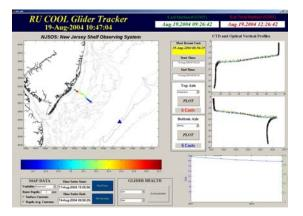
Fig. 5. Phase 3, the Glider GUI. The upper left plot is the track of the Glider color coded temperature. Upper right plot is individual overlayed temperature casts from the last leg. Middle right plot is individual overlayed salinity casts from the last leg. Lower right plot is battery voltage levels since deployment.
