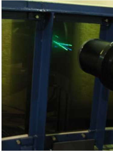
Figure 4. The LDV acquires a velocity profile during the high velocity test in the rotating annular flume. Near-complete entrainment of floc is apparent.
