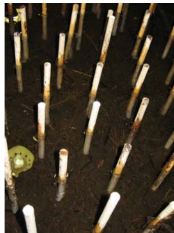
Figure 3. The array of dowels for the “vegetated” run in the racetrack flume, viewed from above. Dowel diameter and spacing was selected to duplicate mean sawgrass stem statistics within Everglades ridges.
