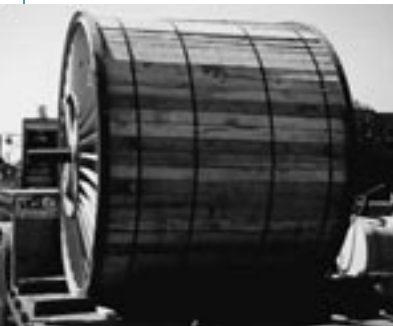
Figure 1 The 11 ton and 10 kilometer spool of LEO-15 electro-optic cable.
