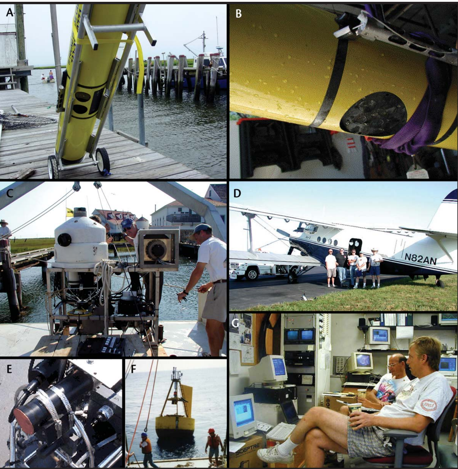
Figure 3. Some examples of now-robust off-the-shelf optical technology during the HyCODE effort that are currently available to oceanographers. (A) A Webb glider ( http://www.webbresearch.com/slocum.htm ) outfitted with an attenuation meter and two backscattering sensors embedded in the belly of the autonomous vehicle. (B) Another Webb glider outfitted with a 2-wavelength backscatter sensor and a fluorometer. (C) A robotic-profiling optical mooring outfitted with absorption-attenuations meters (Wetlabs, Inc.), bioluminescence bathyphotometers, forward-scattering sensors (Sequoia Instruments), and backscatter sensors (HOBI labs and Wetlabs, Inc.). (D) A biplane, one of the world's slowest, outfitted with a hyperspectral, remote-sensing reflectance sensor. The slow speed is ideal for allowing detailed calibration studies. (E) A radiometer (Satlantic) outfitted with a copper shutter. The copper shutters have been demonstrated to be highly effective at minimizing biofouling problems. (F) An optical mooring being deployed by the Ocean Physics Laboratory. (G) Living the dream in the COOL room (Glenn and Schofield, 2003) where scientists can sit and drink coffee while all the data are delivered in near real-time. This capability allows for adaptive sampling (Schofield et al., 2003).
