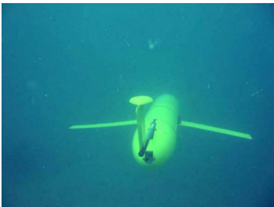
Fig. 3. A Webb Slocum Glider descending into the primordial depths. The science bay is directly behind the wings. The communications package is located in the tail, which is held above the water line when the Glider is at the surface.
