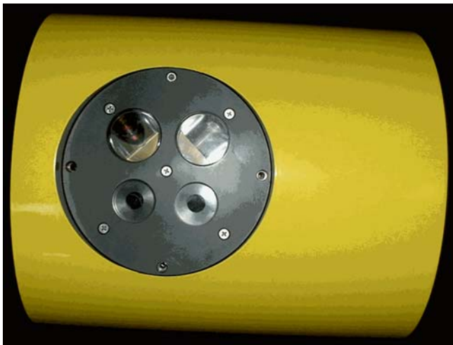
Fig. 3. Hydroscat-2 mounted in the science payload section of the Glider.
