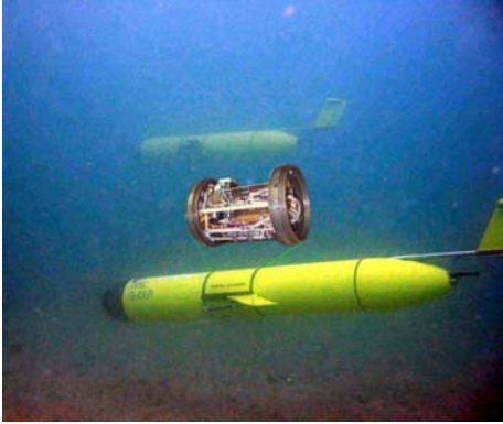
Figure 11 – Brev Buster, a harmful algal bloom detection package as a modular Slocum payload bay.
