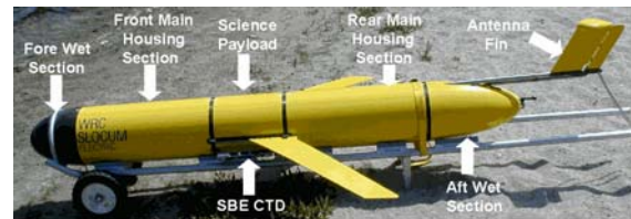
Figure 1 – Overview of Slocum sectional architecture.
